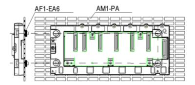
Fasten the rack with four M4, M5, M6 or UNC #6 screws
