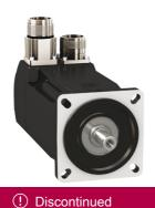
servo motor BMH, Lexium 32, 1.2Nm, 8000rpm, keyed shaft, with brake, IP65, IP67, 16 multiturn encoder, straight
