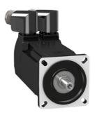
servo motor BMH, Lexium 32, 2.5Nm, 8000rpm, keyed shaft, with brake, IP54, 16 multiturn encoder, 3 phases
