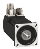
servo motor BMH, Lexium 32, 2.5Nm, 8000rpm, keyed shaft, with brake, IP65, IP67, 16bit encoder, straight, 3 phases
