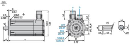
a: Power supply for servo motor brake
