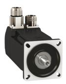
servo motor BMH, Lexium 32, 3.4Nm, 8000rpm, keyed shaft, without brake, IP54, 128 multiturn encoder, straight, 3 phases
