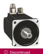
servo motor BMH, Lexium 32, 3.3Nm, 6000rpm, untapped shaft, without brake, IP65, IP67, 16bit encoder, straight
