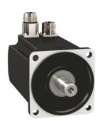
servo motor BMH, Lexium 32, 3.3Nm, 6000rpm, keyed shaft, without brake, IP65, IP67, 16 multiturn encoder, straight
