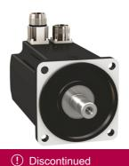
servo motor BMH, Lexium 32, 3.4Nm, 6000rpm, untapped shaft, with brake, IP65, IP67, 128 multiturn encoder, straight
