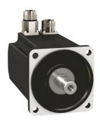
servo motor BMH, Lexium 32, 6.2Nm, 6000rpm, untapped shaft, without brake, IP65, IP67, straight
