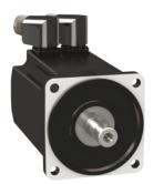
servo motor BMH, Lexium 32, 6.2Nm, 6000rpm, untapped shaft, with brake, IP65, IP67, 16 multiturn encoder
