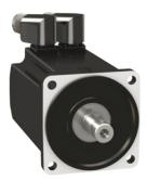
servo motor BMH, Lexium 32, 6Nm, 6000rpm, keyed shaft, with brake, IP65, IP67, 16 multiturn encoder
