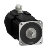
servo motor BMH, Lexium 32, 100Nm, 3000rpm, untapped shaft, with brake, IP20, IP65, 128bit encoder
