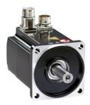
servo motor BMH, Lexium 32, 34.4Nm, 3800rpm, untapped shaft, with brake, IP65, IP67, 128 multiturn encoder
