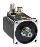
servo motor BMH, Lexium 32, 34.4Nm, 3800rpm, keyed shaft, with brake, IP65, IP67, 128bit encoder, straight
