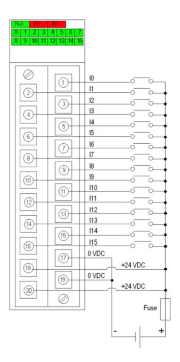
power supply 24 VDC fuse fast blow fuse of 0.5 A
