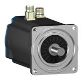
AC servo motor BSH, Lexium 05, 3.39N.m, 4000rpm, keyed shaft, with brake, IP65
