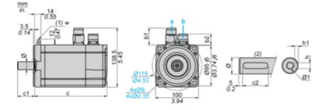
a: Power supply for servo motor brake
