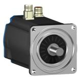
AC servo motor BSH, Lexium 05, 5.5N.m, 4000rpm, keyed shaft, without brake, IP50
