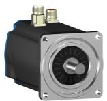
AC servo motor BSH, Lexium 05, 5.5N.m, 4000rpm, untapped shaft, with brake, IP65
