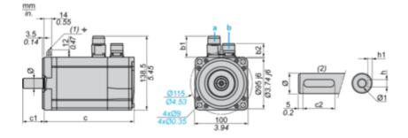
a: Power supply for servo motor brake
