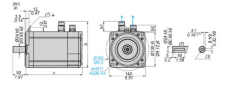
a: Power supply for servo motor brake
