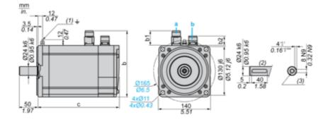
a: Power supply for servo motor brake
