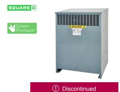
Transformer, dry type, DOE 2016, 150kVA, 3 phase, 208V delta primary, 480Y/277V secondary, 22K, 150C rise
