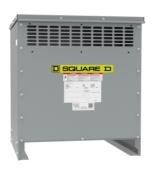
Transformer, dry type, DOE 2016, 30kVA, 3 phase, 480V delta primary, 240V delta secondary, 18M, 150C rise
