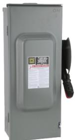
Safety switch, heavy duty, fusible, 100A, 3 wire, 2 pole, 1 neutral, 30HP, 240VAC, 250VDC, NEMA 3R, bolt on hub provision
