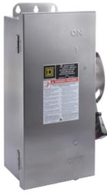
Safety switch, heavy duty, fusible, 60A, 3 wire, 3 pole, 15hp, 240VAC/250VDC, NEMA 4, 4X, 5, 304 stainless steel
