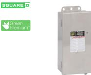
Safety switch, heavy duty, fusible, 30A, 600VAC, 600VDC, 3 poles, 20hp, NEMA 4, 4X, 5, 304 steel, Crouse-Hinds
