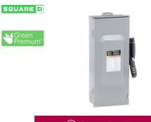
Safety switch, heavy duty, fusible, 100A, 4 wire, 3 pole, 1 neutral, 100hp, 600VAC/DC, NEMA 3R, bolt on hub provision
