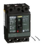
Circuit breaker, PowerPacT H, 80A, 3 pole, 600VAC, 25kA, lugs, thermal magnetic, 80%
