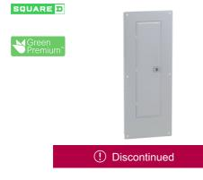
Load center, Homeline, 1 phase, 40 spaces, 80 circuits, 200A convertible main breaker, PoN, NEMA1, gnd bar, bulk pack
