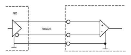
The reference pulses are supplied via two of the signal inputs, either as pulse/ direction signals or as A/B signals. The other signal inputs have the functions "power amplifier enable/pulse blocking" and "step size switching/PWM motor current control".
