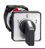
Complete cam switch, Harmony K1, K2, cam changeover switch, 16mm or 22mm, plastic, 2 poles, position 0, 60degrees, 10A, 30x30mm, marked 1 0 2
