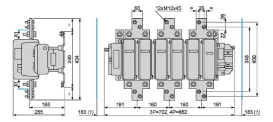
(1) Minimum distance required for coil removal.
