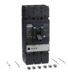
Circuit breaker, PowerPacT L, 400A, 3 pole, 600VAC, 25kA, lugs, MicroLogic 3.3, 80%
