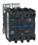
IEC contactor, TeSys Deca, nonreversing, 125A resistive, 4 pole, 2 NO and 2 NC, 48VDC coil, open style
