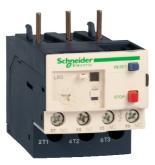
Thermal overload relay, TeSys Deca, 690VAC, 0.1 to 0.16A, 1NO+1NC, class 10A, for unbalanced loads
