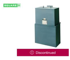
Unit substation, Mini Power-Zone, plug on, 15kVA, 3 phase, 480V primary, 208Y/120V secondary, 25kA, C
