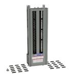
Panelboard interior, NQ, main lugs, 225A, Al bus, 72 pole spaces, 1 phase, 3 wire, 240VAC, 48VDC
