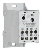
Power distribution block, Linergy, enclosed, 2 line, 8 load, 335A Cu, 270A Al, 600V, Al lug, panel
