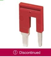
Reduction bridge screw to spring, Linergy TR terminals blocks, for conecting 35mm<sup>2</sup> screw to 2.5/4mm<sup>2</sup> spring terminal, red
