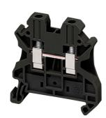
Terminal Blocks, Linergy, feed through, 30A, 600V, screw termination, 2 points, 26AWG to 10AWG, black
