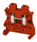
Terminal Blocks, Linergy, feed through, 30A, 600V, screw termination, 2 points, 26AWG to 10AWG, red
