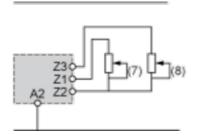
7 Off-delay adjustment (tr) (contact 15/16 closed).8 On-delay adjustment (ta) (contact 15/18 closed).
