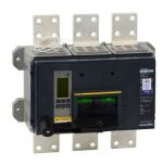
Circuit breaker, PowerPacT R, 1000A, 3 pole, 600VAC, 65kA, busbar, Micrologic 6.0P, 100%, modbus
