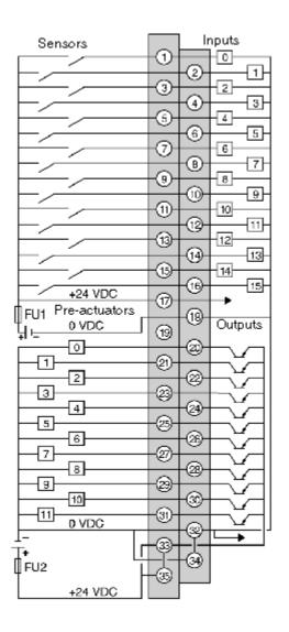
FU1 = 0.5A fuse with rapid fusion. FU2 = 6.3A fuse with rapid fusion.
