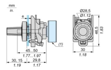
e: panel thickness: 1 to 6 mm / 0.04 to 0.24 in. (1) Potentiometer not included
