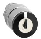
Head for key selector switch, Harmony XB4, 22mm 3 positions spring return, key 455, chromium plated metal bezel
