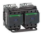
Reversing Contactor, TeSys Deca, 3P(3NO), AC-3/AC-3e, <=440V 80A, 120V 60HzAC 50/60Hz coil, screw clamp terminals
