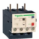
Thermal overload relay, TeSys Deca, 690VAC, 0.1 to 0.16A, 1NO+1NC, class 10A, for unbalanced loads
